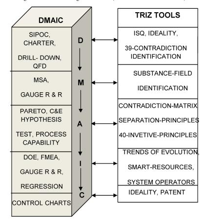
Figure 2 Integrated model of Six Sigma and TRIZ (see online version for colours)
