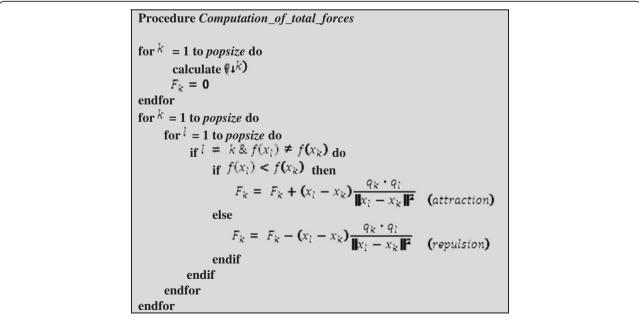
Figure 3 The procedure of calculating total forces.
