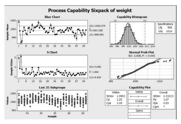
Fig. 4 Test of normality, control charts of present data and calculations of Cp and Cpk
