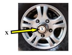
Fig. 3 Alloy wheel in assembly,  $X = \text{center hole diameter of } \phi 50.000^{(\pm 0.050)}$
