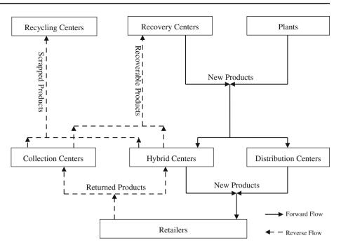
Recovered products are inserted in the forward network and are considered identical to new products.
