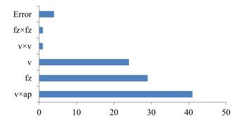
$\textbf{Fig. 10} \ \ \text{The effect of machining parameters on the SR}$
