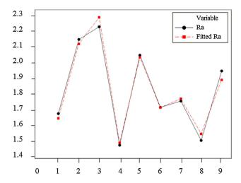
Fig. 6 Predicted versus actual surface roughness
