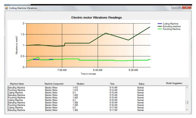
Fig. 10 Form for a typical output of vibration data from electric motors
