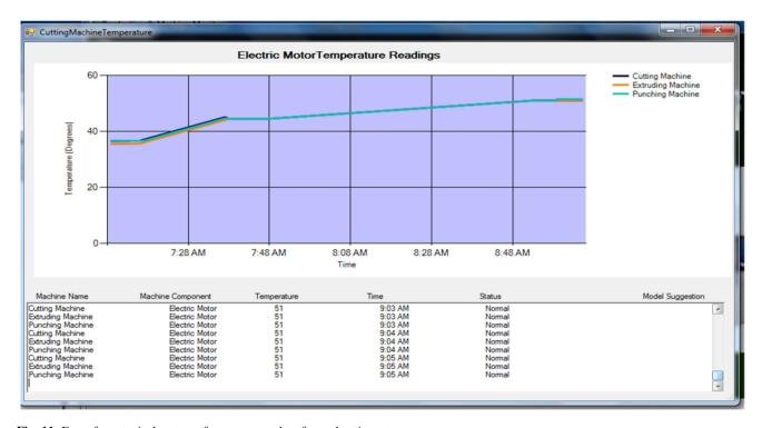
Fig. 11 Form for a typical output of temperature data from electric motors
