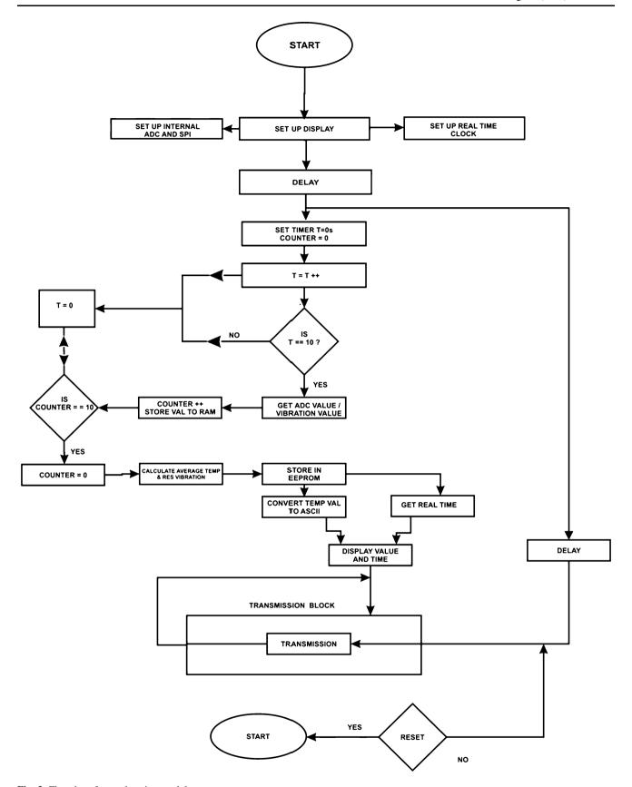
Fig. 3 Flowchart for workstation module
