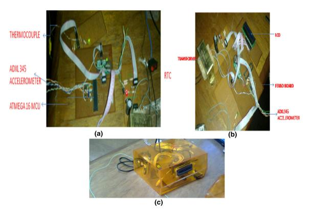
Fig. 6 Workstation hardware components on board at point of testing and the assembled hardware
