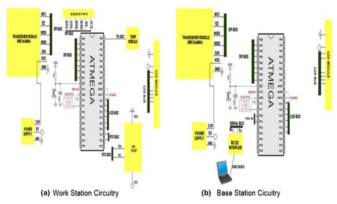
Fig. 5 Circuit diagram for the developed work station and base station
