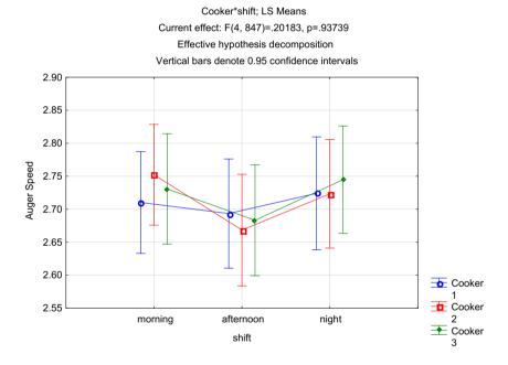
press. It is possible that the speed of this device is affecting the density of the product as it enters the press system (which has its own fixed-speed auger). In turn, this suggests that operator judgements at the unloading of the cooker may be affecting the process.
