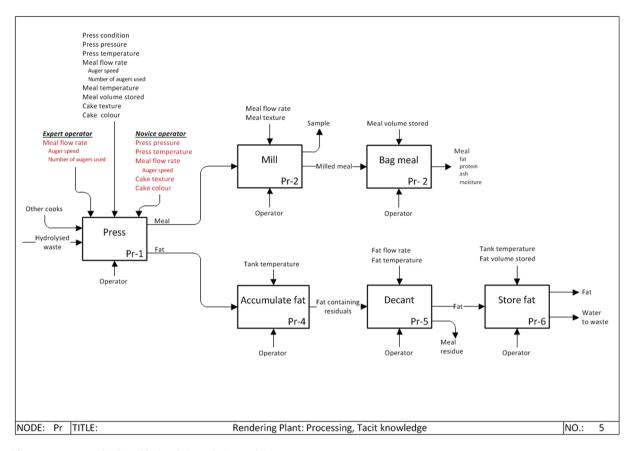
Fig. 10 Press process with identified tacit knowledge variables
