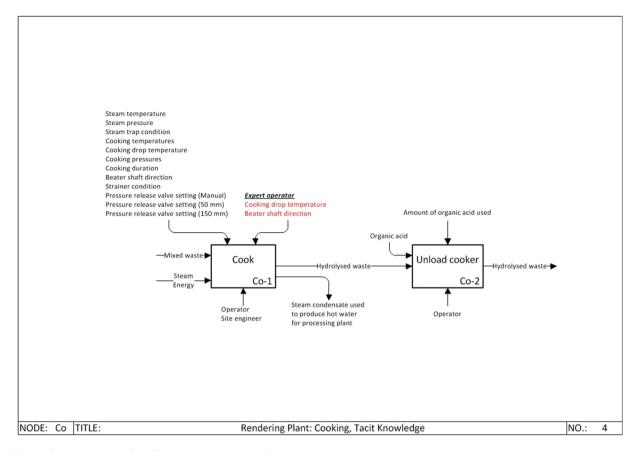
Fig. 9 Cooking process with identified tacit knowledge variables
