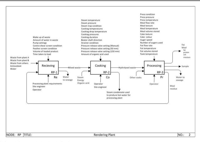
Fig. 3 Rendering process broken down by function
