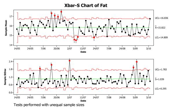
Fig. 6 Rendering plant control chart analysis
