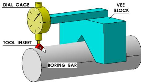
Fig. 7 Schematic diagram of tool insert setting V-Block
