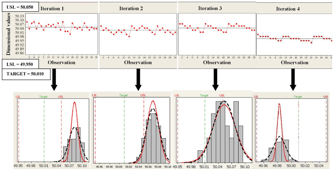
**Fig. 6** Process capability analysis depicting run charts and histograms of Iterations 1, 2, 3 and 4
