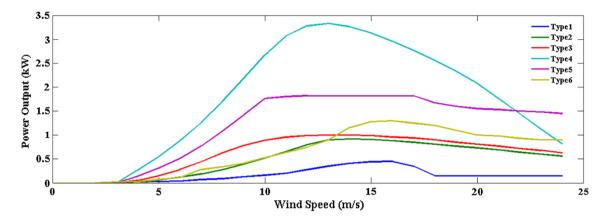
Fig. 5 Wind turbine power curves (the symbols represent data sampled from the power curve graphs given by the manufacturer)
