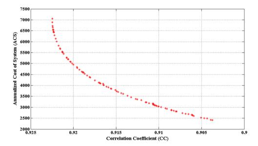
evolution of the 3D Pareto front can be observed in Fig. 13. When a pre-specified iteration count ( $N = N_{\rm max}$ ) is reached, MOPSO is terminated.  $N_{\rm max} = 200$  and a population size of  $N_{\rm pop} = 200$  are considered.
