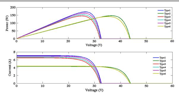
Fig. 7 P-V and I-V curves for different PV modules
