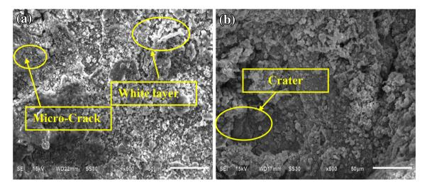
Fig. 10 a, b SEM micrograph of drilled surface
