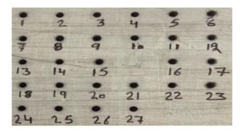
Fig. 3 Specimen after EDM drilling
