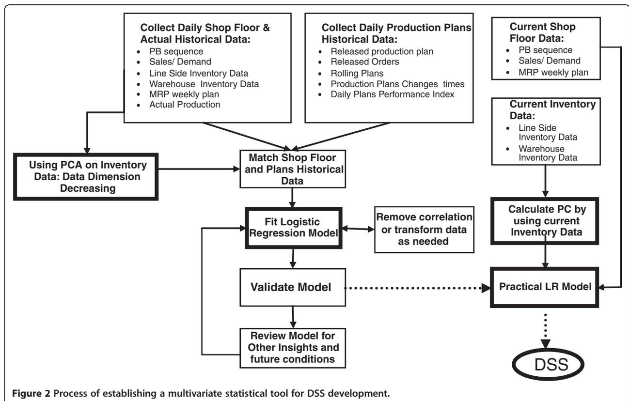
**Figure 2** Process of establishing a multivariate statistical tool for DSS development.
