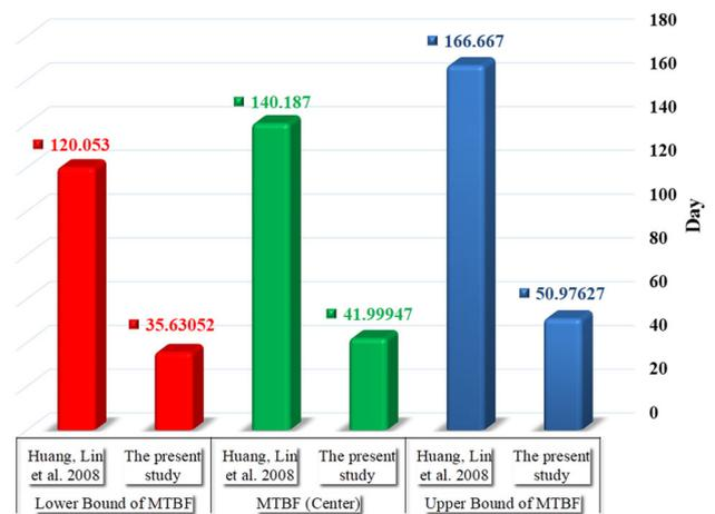
**Fig. 7** The comparison of MTBF for the two models
